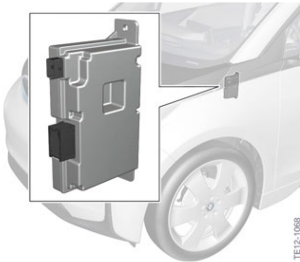
KAFAS control unit
